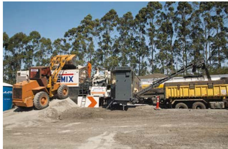
The high performance Wirtgen cold recycling mixing plant KMA 220 has an impressive mixing capacity of up to 220 t/h when producing high-quality cold mix from recycled construction materials.
